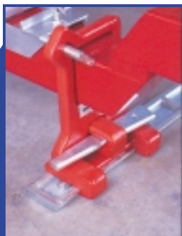
Fast locking wedges secure the vehicle to the floor rails without bolts.
