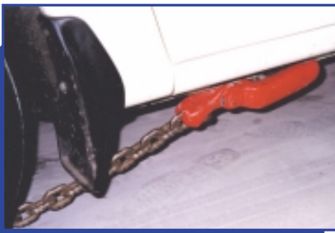
Wedge clamp for light repairs. Start pulling in one minute
