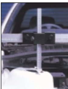
Overhead Measuring - Used to check strut towers and upper body points
