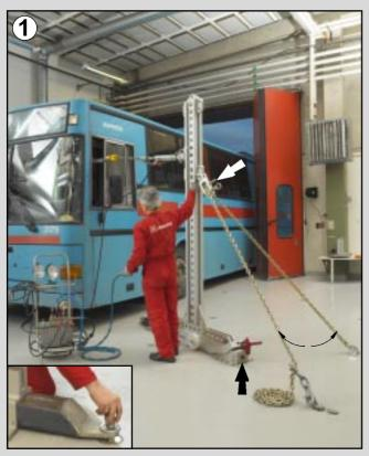
The floor anchoring is exceptional when it comes to repair of minor damage, as for this coach. In this case the cab tower is fixed with a nose bracket directly in the expander hole at the front and with chains at the rear. The tower is pretensioned with an impact wrench (see lower arrow). The pulling angle is quickly adjusted sideways and the tower locked into position with a pin (see upper arrows).
