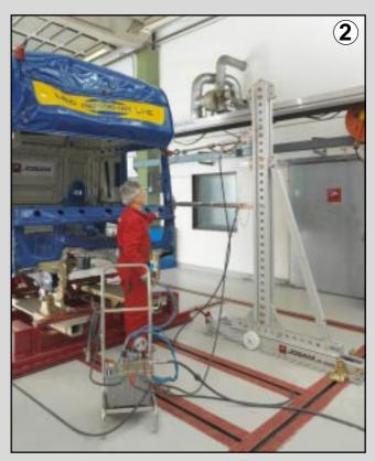
The conventional anchoring system fixes the cab tower into I-beams which have been installed in the shape of a "cab square" or as frame straightening rails.
