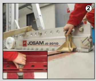
The I-beam anchoring fits in the same anchoring holders as JOSAM frame press. With a simple twist the cab tower is fastened into the I-beam in the workshop floor. Of course, our JOSAM cab bench also fits in the I-beams.
