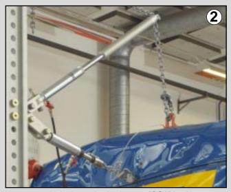
No matter which alternative is chosen, JOSAM cab tower can be utilized for many different repair jobs, thanks to its versatility. Here, for instance, a straightening job with advanced vector pulling is performed at 3-4 meters' height.
