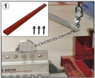
The nose bracket kit allows the trolley to be locked directly to the cab bench for cab repair jobs.
